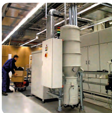
Cyclonic filter FZ-1003 with 100 Litre collection container
