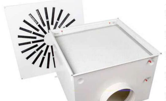
Hepa Terminal Box is a terminal filtration device in which terminal hepa filters insalled. It consists of a static pressure box, HEPA filter and diffuser.
